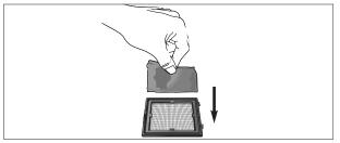
**6.** Replace the filter cover. Insert the tab on the end of the filter cover into the filter cover opening and press the filter cover into position.
